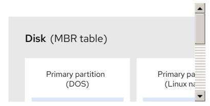
As this figure implies, there is a difference between primary and logical partitions - there can be only up to four primary and extended partitions, but there is no fixed limit to the number of logical partitions that can exist. However, due to the way in which partitions are accessed in Linux, no more than 15 logical partitions can be defined on a single disk drive.
