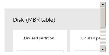
As the previous diagram shows, the partition table is divided into four sections of four primary partitions. A primary partition is a partition on a hard drive that can contain only one logical drive (or section). Each section can hold the information necessary to define a single partition, meaning that the partition table can define no more than four partitions.
